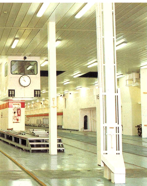
Train deck with shunting central above clock.
