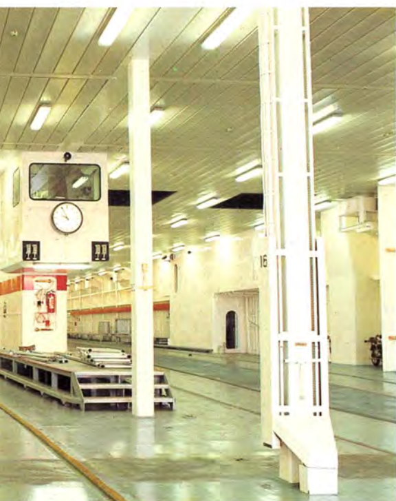
Train deck with shunting central above clock.
