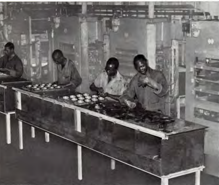
Rubber Engineering & Products. Formvulkanisering af såle og hæle. Rubber Engineering & Products. Moulding of soles and heels.
