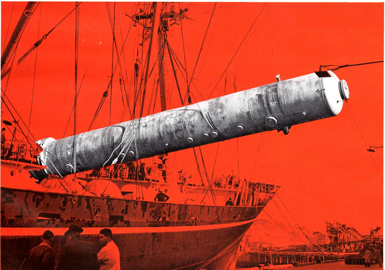
Sværvægtsgods, en pulpkoger på 60 tons, losses med skibets egne grejer. Heavy weight goods, a pulp boiler of 60 tons, being discharged by the ship's own derricks.
