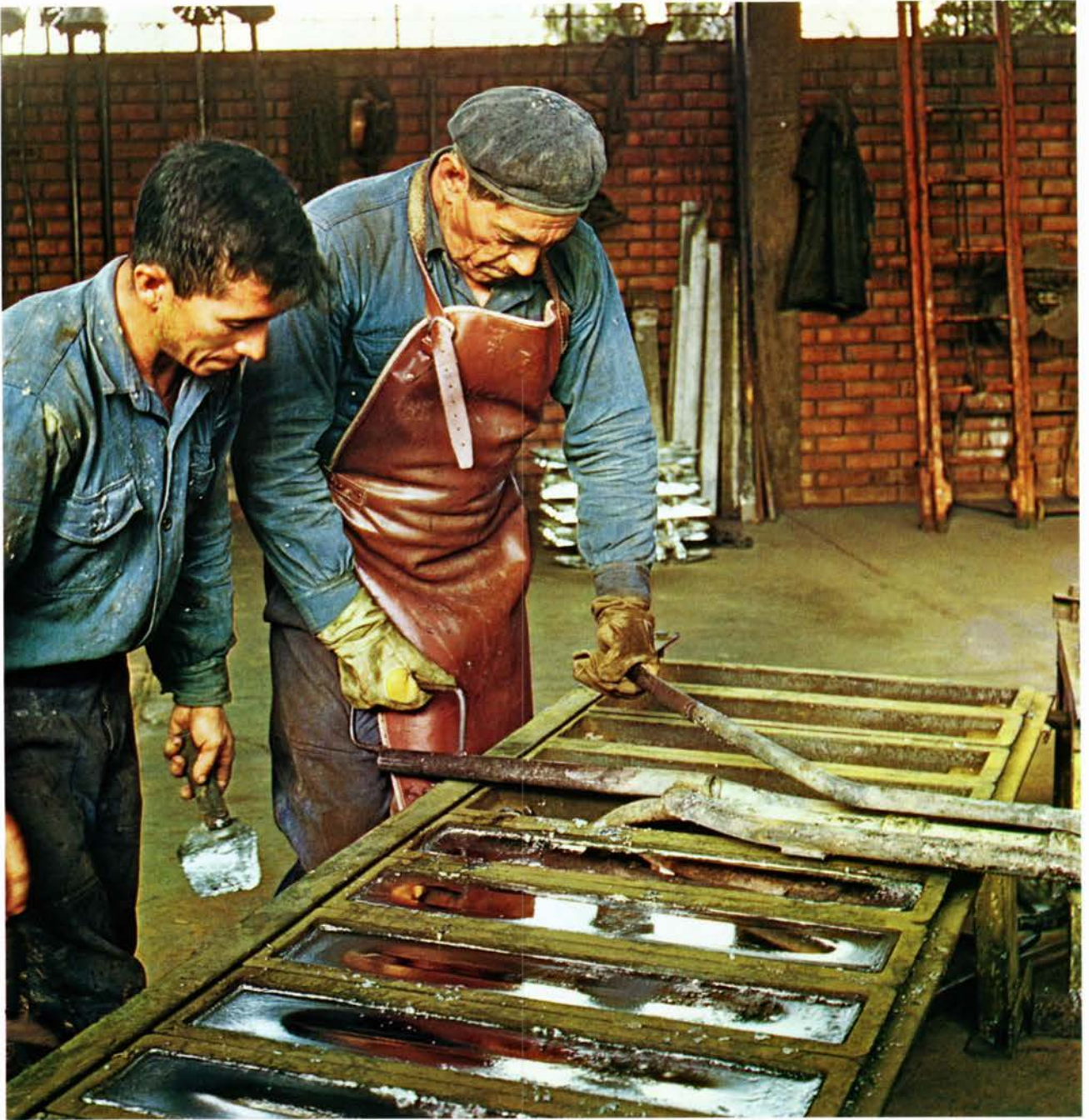
Cali. Antimonbly udstøbes i metalblokke. Cali. Antimonial lead being casted into ingots.
