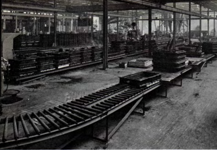
Mekaniseret støberi. Rullebaner med formkasser. Mechanized foundry. Rolling way with moulding boxes.
