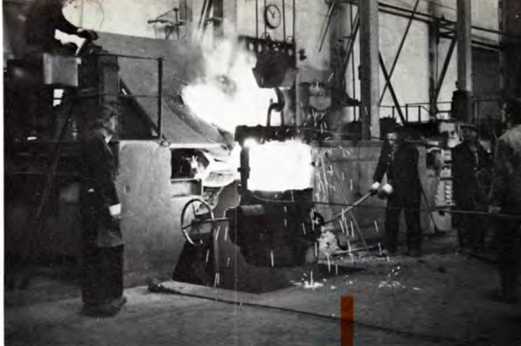
1 ton elektrisk smelteovn. 1 ton electric melting furnace.
