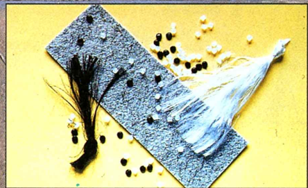
Above: Granulate, fibre and finished product. Main picture: Fibertex was used in the construction of a runway at Tirstrup Airport, Jutland
