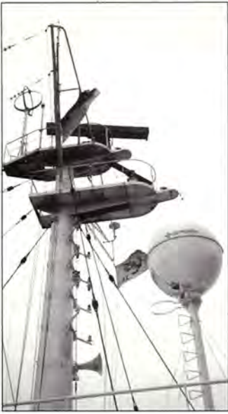
The Sperry SATCOM aerial handles ship-to-shore data transmission.
