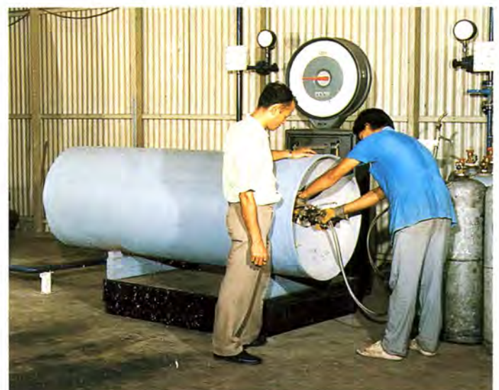
Due to the hot and humid climate, Thailand has a significant demand for refrigeration and airconditioning. ICI refrigerants are liquified gases requiring special storage facilities. Deliveries to customers are being effected in drums or cylinders, filled at EAC (Thailand)'s warehouse.
