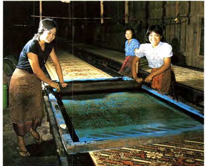
Thailand's textile industry varies from large modern automated plants to small factories. Here ICI dyestuffs are being applied by hand screen onto cotton.
