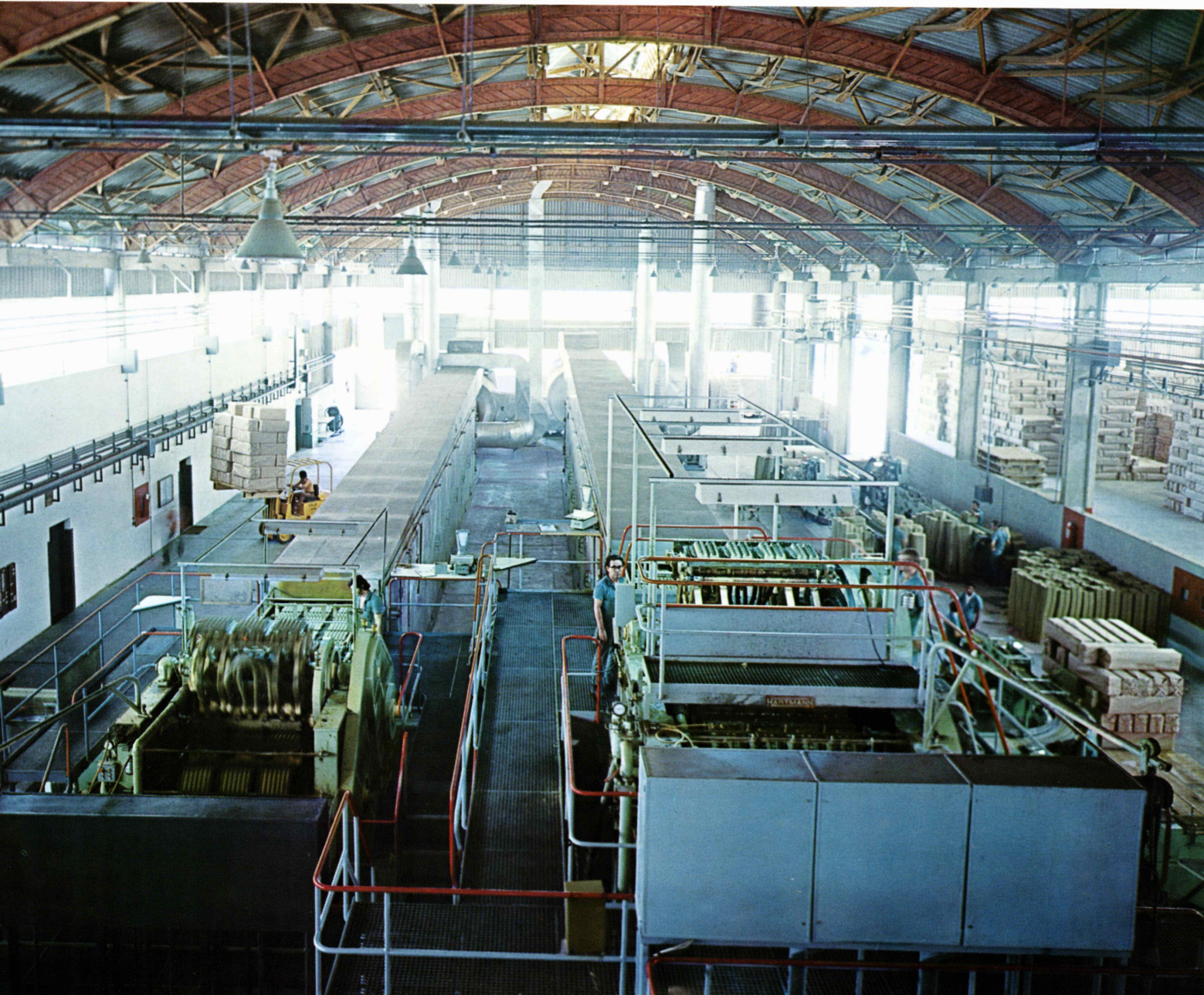
Sorocaba. View of the factory halls. In the foreground the two moulding machines, in the centre drying tunnels, and to the right in the background stores.
