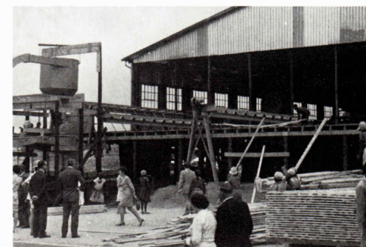
New Scotland Development. Enden af savmøllen med transportbånd og til venstre en flishugger. New Scotland Development. End of wet mill, showing green chains, and (on the left) chipper.
