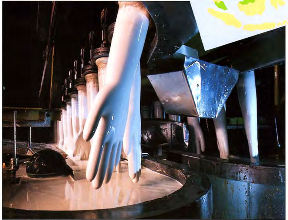
The "hands" pass through dip tanks
